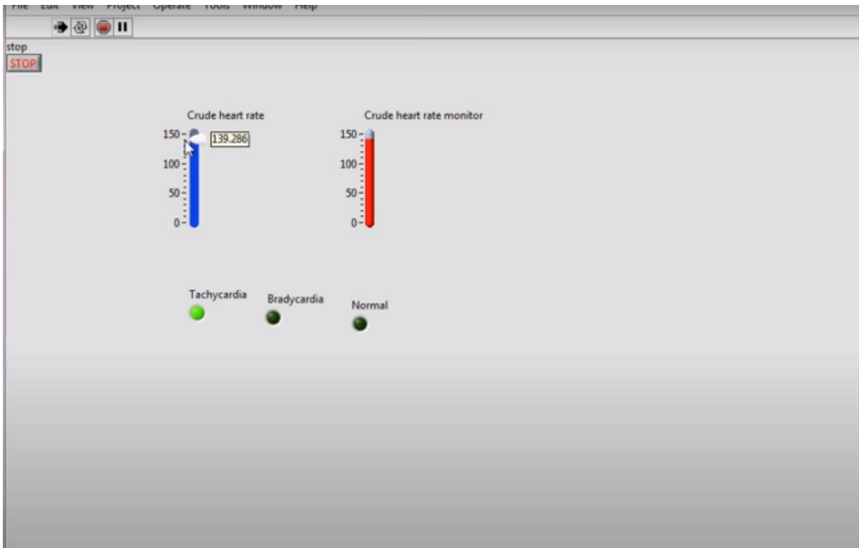
Fig 4.1.3 Real-time output in LabView for various body conditions
