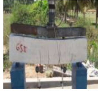
Fig 3: Crack pattern of the beam
